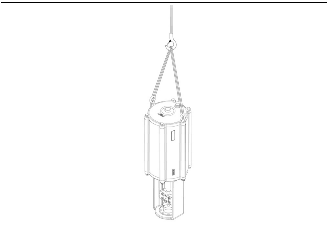
Fig. 5 Lifting the actuator.
