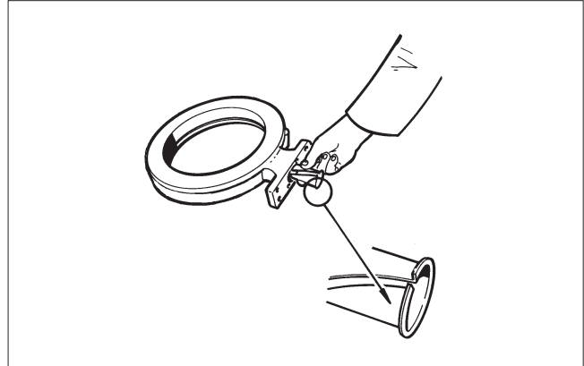
Fig. 16 Mounting the standard bearings
