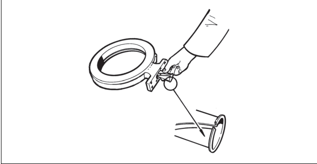
Fig. 17 Mounting the standard bearings
