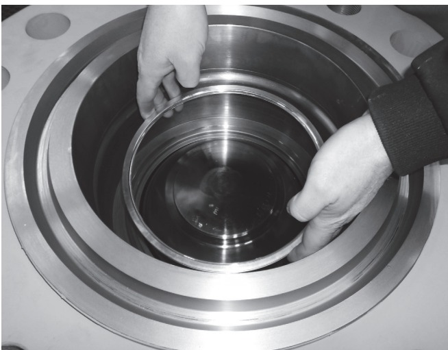
Fig. 24 Replace the metallic seat ring (321)
