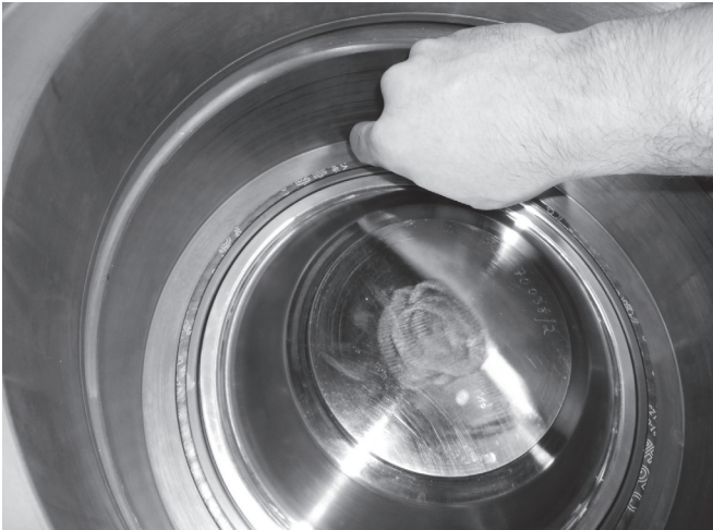
Fig. 23 Remove the sealing ring (304)
