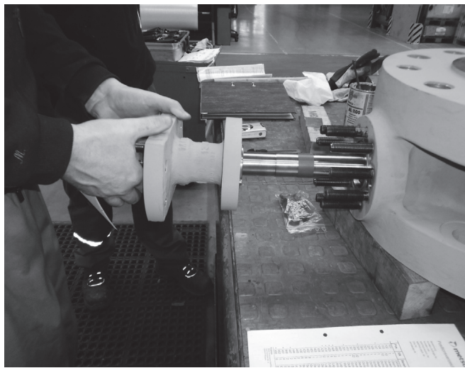
Fig. 32 Remove the extension (102)
