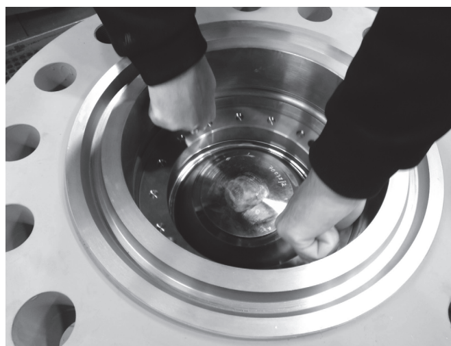
Fig. 22 Remove the inner seal lock ring (301)
