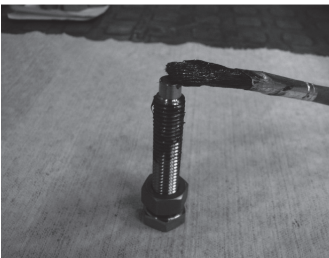
Fig. 25 Lubricate the screws with Molykote
