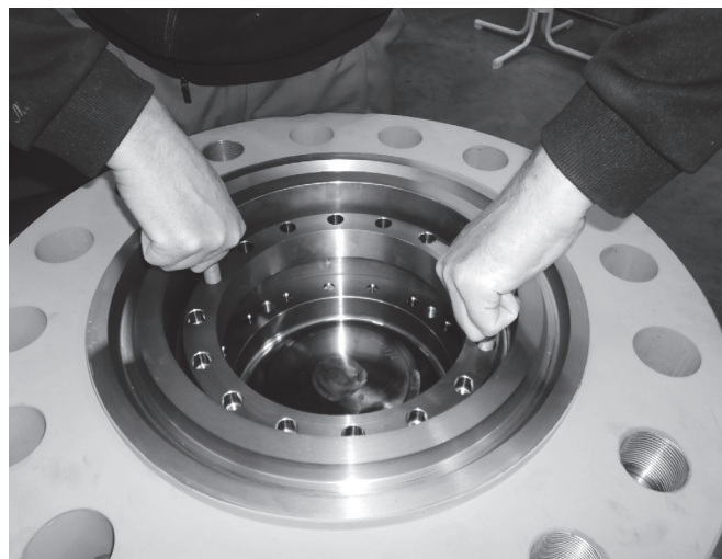
Fig. 21 Remove the outer seal lock ring (303)
