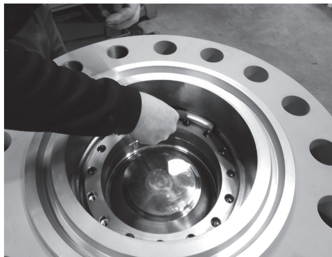
Fig. 20 Demount the retaining ring (310)
